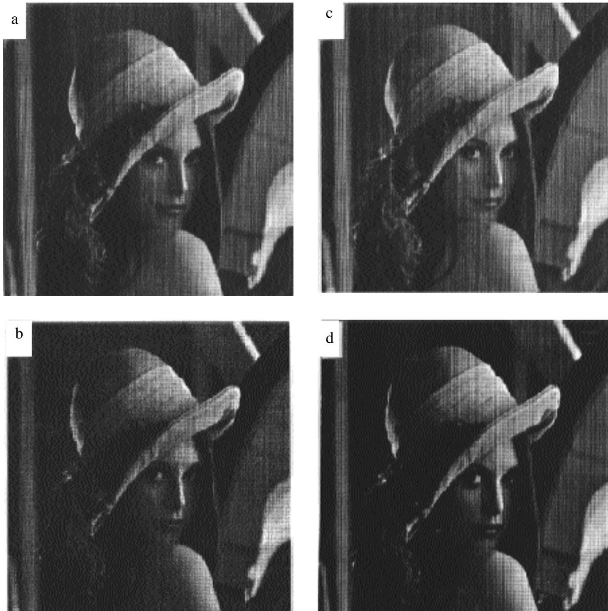
Figures 1a-1d. Dramatic variation in inkjet quality of plain papers printed with the Hewlett-Packard Deskjet printer.
