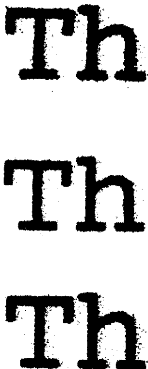
Figure 4. "Th" characters printed with Hewlett Packard's DeskJet 540 printer using: A) 51626A dye-based ink (top), B) Pigment 1 ink (middle), and C) Pigment 2 ink (bottom)
