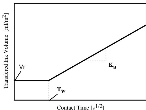
Figure 1. Typical dynamic sorption curve of water based ink absorption
