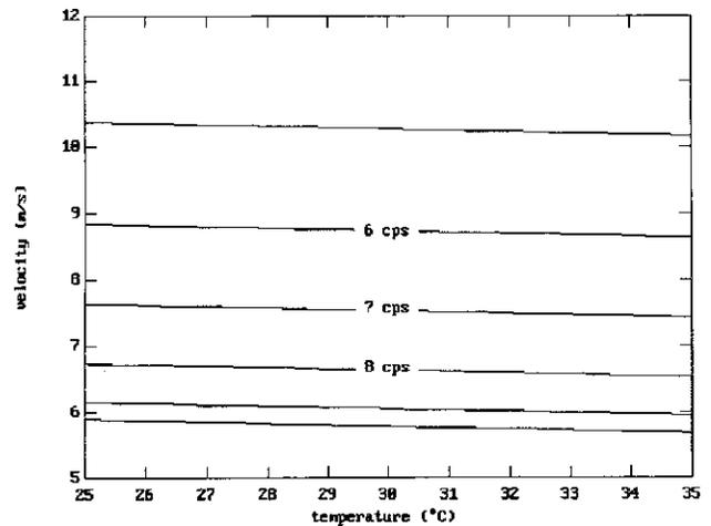
Figure 5. Drop velocity versus temperature for various ink viscosities.
