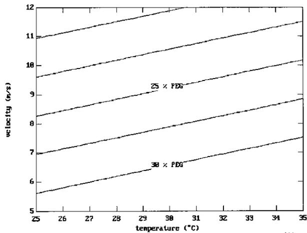
Figure 3. Velocity versus temperature for various PEG concentrations.
