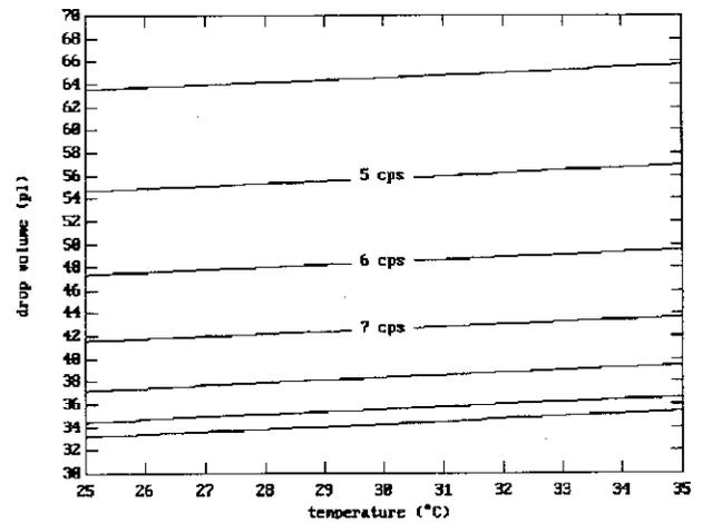
Figure 4. Drop volume versus temperature for various ink viscosities.
