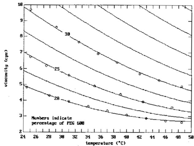
Figure 1. Viscosity versus temperature for various PEG concentration.
