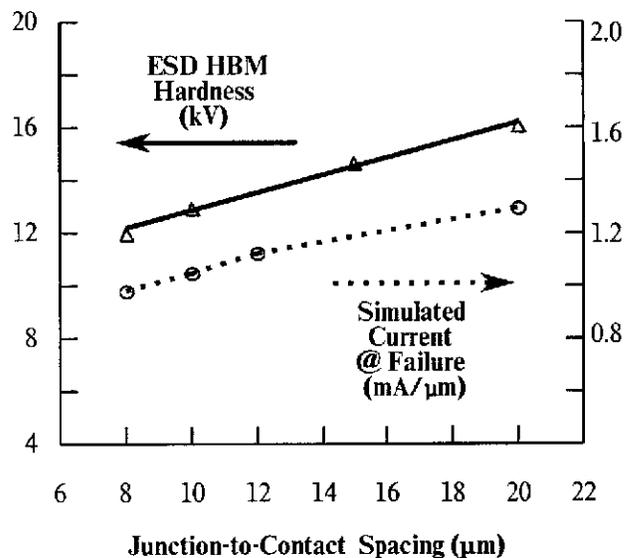
Figure 4. Measured ESD human-body-model hardness and simulated DC current for which Al/Si eutectic temperature is reached at the drain contact.
