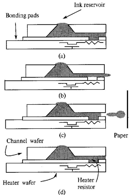
Figure 1. Cross-section of a side-shooter drop ejector during a firing sequence at time steps: (a) 0 s. (b) 3 s. (c) 20 s. (d) 200 s.
