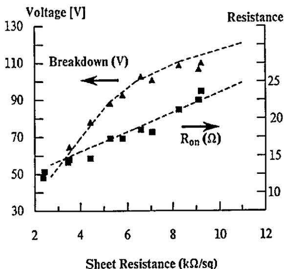
Figure 3a. Driver breakdown voltage and on-resistance dependence on drift sheet resistance. Dotted line are simulation results, symbols are experimental data points.
