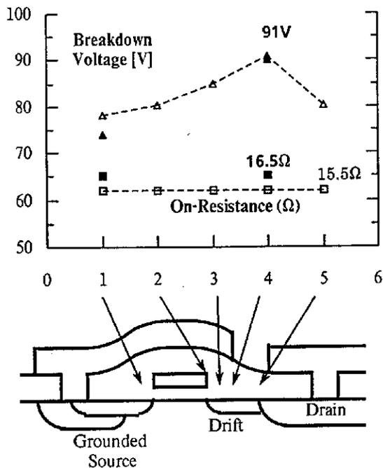
Figure 3b. Driver breakdown voltage and on-resistance dependence on aluminum field plate extension over the drift region. Open symbols and dotted lines are simulation points, closed symbols are experimental data points.
