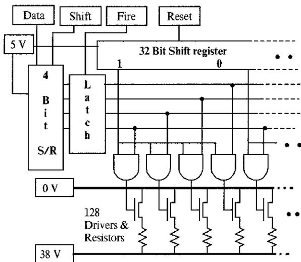
Figure 2. Thermal ink jet logic-on-board chip architecture for a 300 spi, 128 element printhead.
