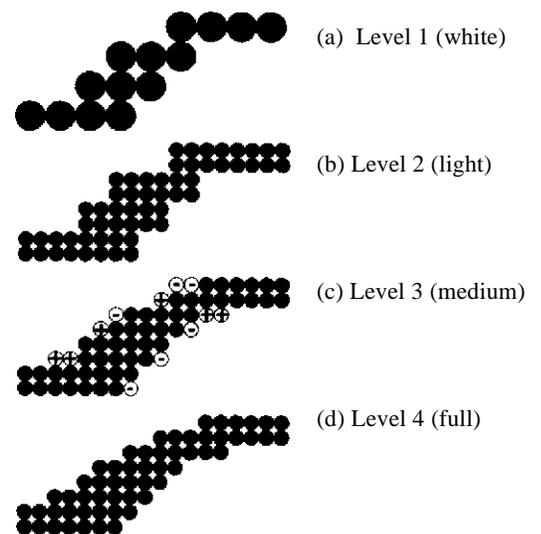
Figure 1. REt processing sequence: (a) original  $300 \times 300$  dpi data, (b) simple  $2 \times$  expansion from 300 dpi to 600 dpi, (c) REt algorithms applied, (d) 600 dpi image after REt
