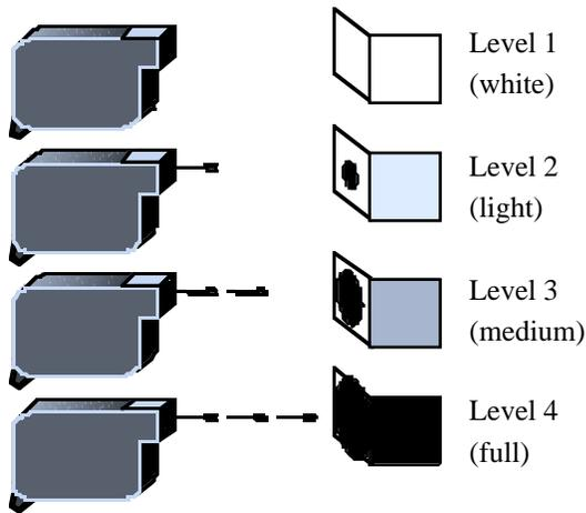
Figure 2. C-REt uses small drop volume and multiple drops at 300 dpi to achieve 4 levels per pixel
