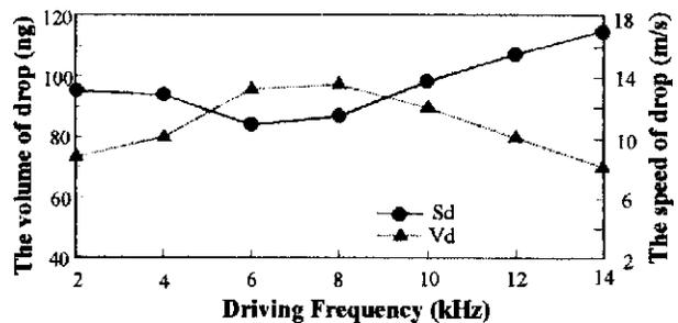
Figure 2. The Relationship between Driving Frequency and the Speed of Drop (Sd), the Volume of Drop (Vd)
