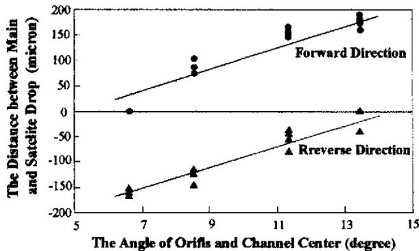
Figure 4. The Relationship Angle between orifice and channel center versus Distance between main and satellite dot on a printed matter.
