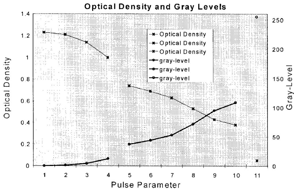
Figure 3. Optical density range and grey-level assignment resulting from drop volume modulation.
