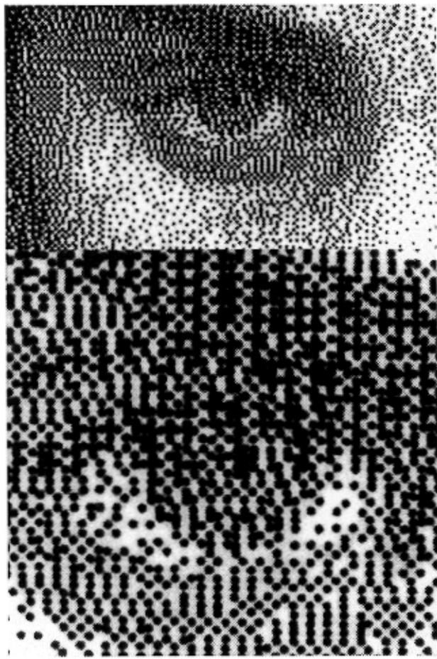
Figure 4. Photomicrograph of fixed spot printing using the same printhead and original image as was used in Figure 4
