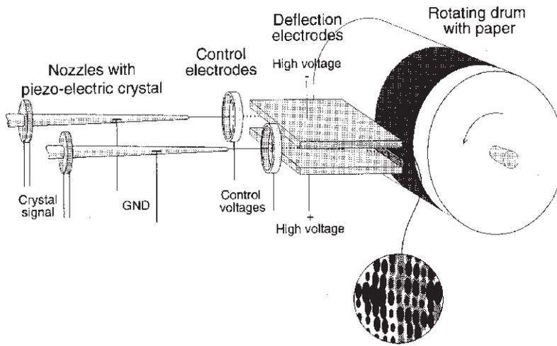
Figure 2. Principle of the continuous inkjet printer using dual ink densities.
