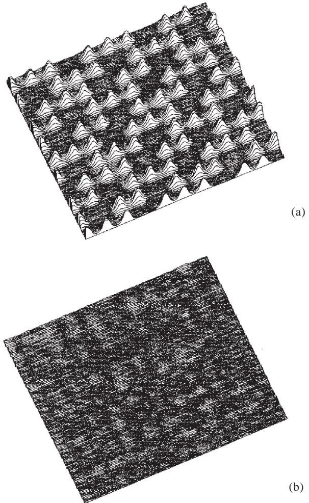
Figure 8. Three dimensional plots of the 5% density print samples showing the local variations in density over  $10 \times 10$  pixels from (a) single ink density printing and (b) dual ink density printing.
