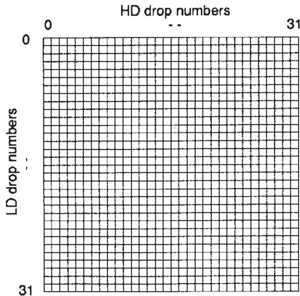
Figure 3. Test image for the measurement of all possible combinations of true density levels printed with drop numbers from 0-31 of the high density (HD) ink together with 0-31 drops of the low density (LD) ink.
