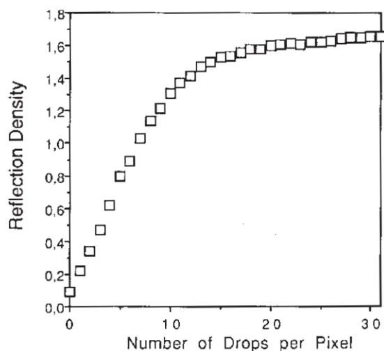
Figure 1. Reflection density versus the number of drops deposited in every pixel
