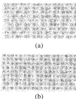
Figure 5. Magnification of prints showing differences in dot placements. In (a) the one-drop dots are misplaced because of the air resistance acting on the single flying drop, whereas in (b) this effect has been compensated for by "firing" the single drops at an earlier time point.
