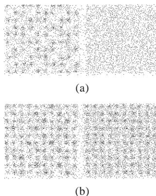
Figure 6. Magnification of print samples with reflection density levels of (a) 5% and (b) 10%. The samples to the left in both (a) and (b) are printed with only one ink density, whereas the ones on the right are printed with dual ink densities.
