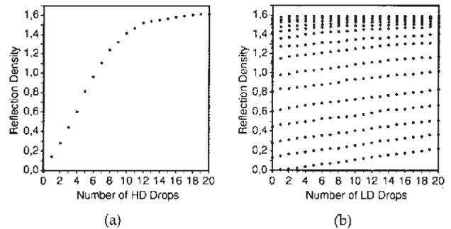
Figure 4. Diagram of the measured reflection density versus the number of drops of (a) HD ink, and (b) "LD ink Con top" of ground levels of HD ink for drop numbers from 0 to 20.
