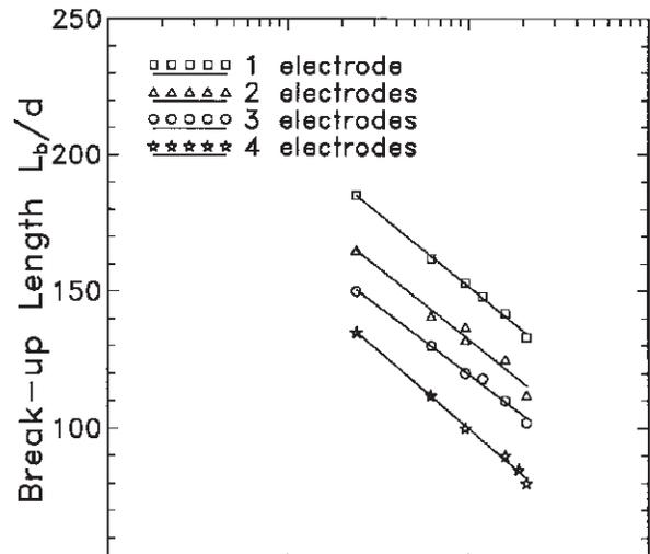
Figure 6. Break-up length as a function of the frequency of the driving voltage for 1 and 4 ring electrodes
