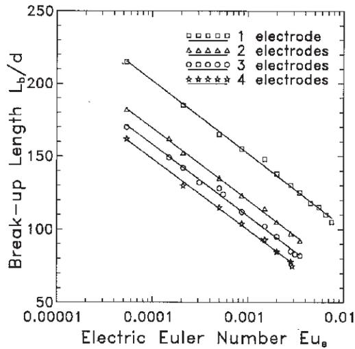
Figure 2. Break-up length with 1 to 4 ring electrodes as a function of the electric Euler Number  $Eu_e$ .
