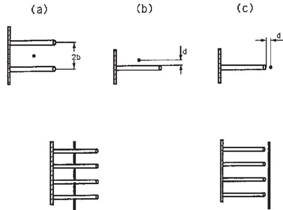
Figure 4. Asymmetrical 4 electrode geometries. Top views (upper half of the figure) and side views (lower half) of the jet/electrodes arrangement (the left side view is common to cases [a] and [b]).
