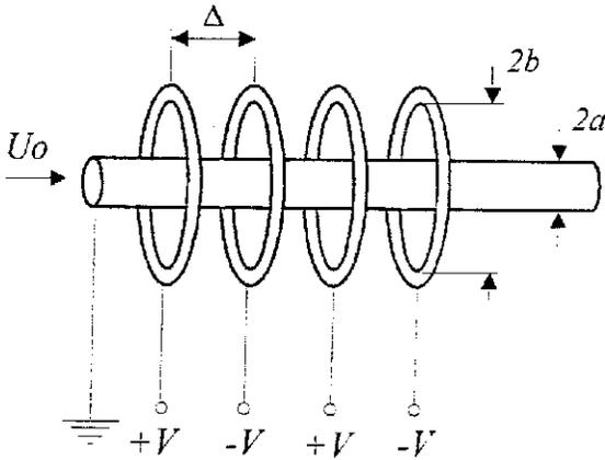
Figure 1. Schematic view of the stimulation ring electrodes around the liquid jet (note the 180° phase shift of their electrical potential).
