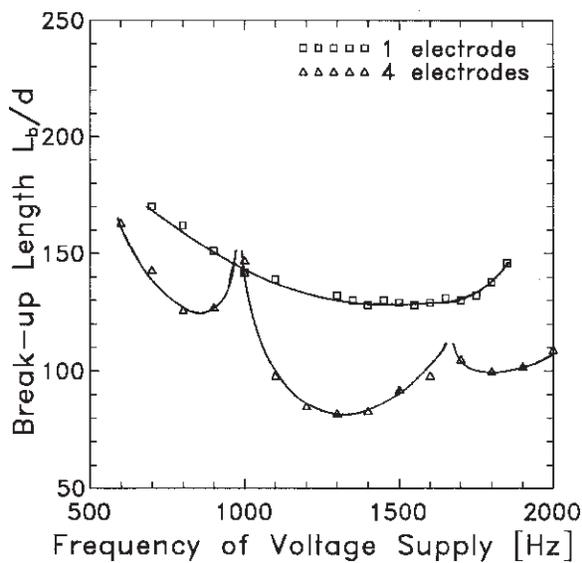
Figure 5. One set of parallel wire electrodes: Break-up length as a function of the electrical Euler number  $Eu_c$  for 1 to 4 electrodes
