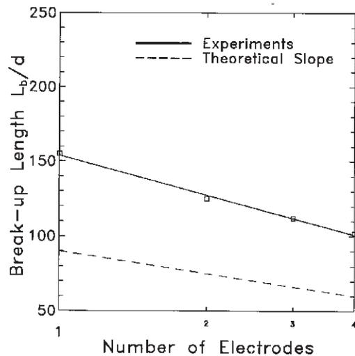
Figure 3. Break-up length as a function of the number of used ring electrodes for  $Eu_e = 10^{-3}$ .
