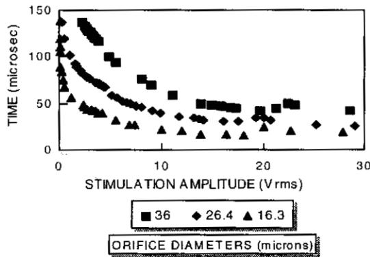
Figure 3. Graph of breakup time versus stimulation amplitude for conditions shown in table 3
