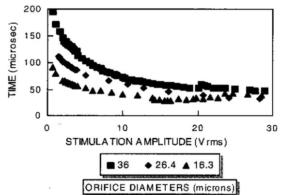
Figure 1. Graph of breakup time versus stimulation amplitude for conditions shown in table I.
